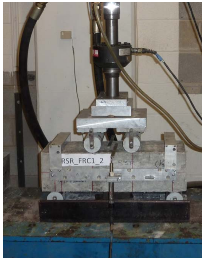
Figure 4.4. Residual strength ratio testing.
