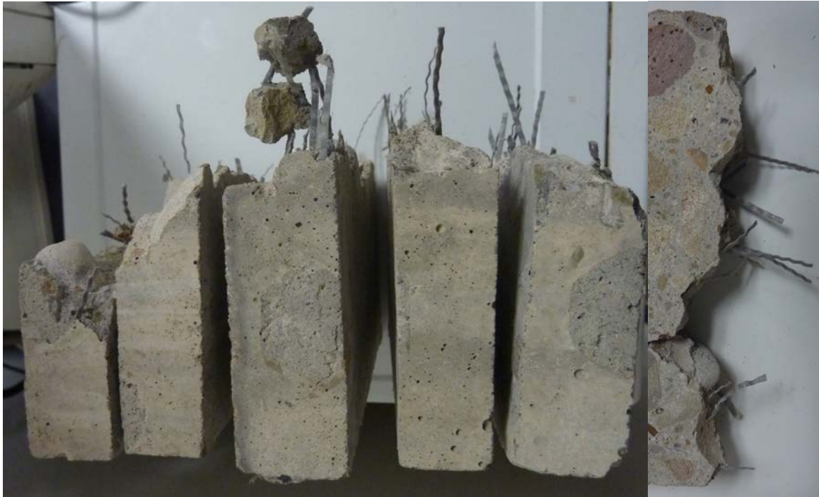
Figure 5.32. Pictures of F2 fiber (Enduro 600) after fatiguing with 10 million load cycles.
