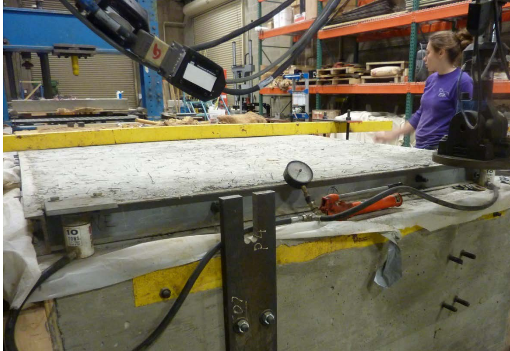
Figure 3.31. Slab cracking procedure.
