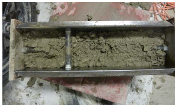
Figure 3.17. Preparation of an FRC beam specimen is in progress.
