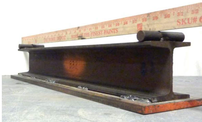
Figure 3.5. The top I-beam in B ALT setup.
