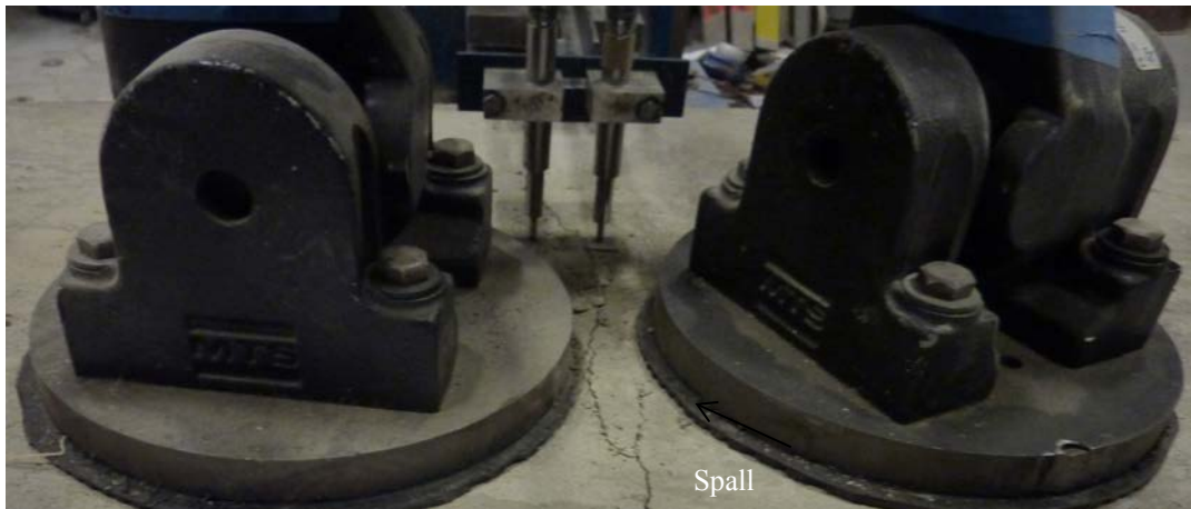
Figure 5.53. Picture of the crack after 600,000 load cycles.
