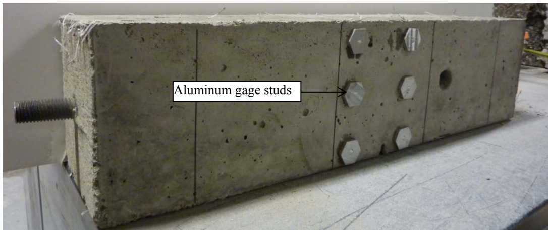
Figure 3.19. Aluminum gage studs for measuring crack width.
