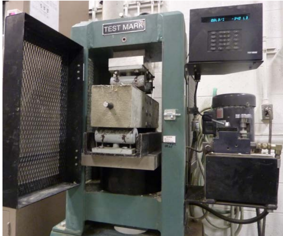
Figure 3.20. Cracking procedure for the beams used for B_{ALT} .
